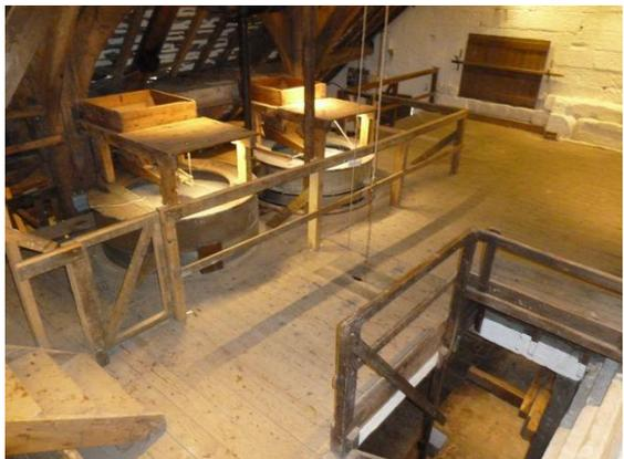
Specialist millwrights were engaged for a full overhaul of the machinery, with some cracked sections being recast to enable safe running of the waterwheels. Grain can now be milled for flour, a major visitor attraction. New barriers were installed to allow millers to operate safely.
